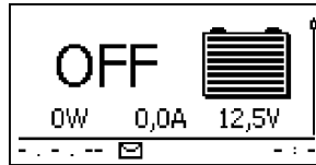
Fig. 4: Display after switching on the external battery fuse
