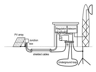
The connection between modules and charge regulator should be shielded. All metal parts should be grounded. Lightning rods can help to protect from voltage spikes but they should not shadow the modules at any time.
