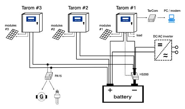
In a photovoltaic system several PowerTarom regulators can charge a battery simultaneously. Please note the following notes for an optimal installation:
