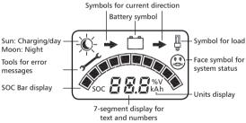
The display modes change automatically. The changing can be stopped and released with the left key. The bar display shows the actual battery level (SOC = state of charge) of the battery in each window. If the regulator is set to voltage control, the SOC bar display does not appear and the battery voltage value replaces the SOC percentage value!
